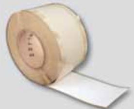
Cover Strip is exclusively tested and designed for use on Carlisle Sure-Flex PVC and KEE HP membranes only and is available in white, gray, and tan 6"-wide by 100'-long (152 mm by 30.5 m) rolls. Performance of PVC PS Cover Strip is not guaranteed if used on other manufacturers' membranes. PVC PS Cover Strip is used to strip in flat metal edgings (e.g. drip edge).
